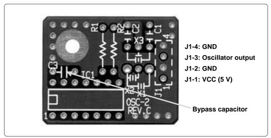
Figure 5.1 External view of the oscillator board (OSC-2) and connector pin assignment
